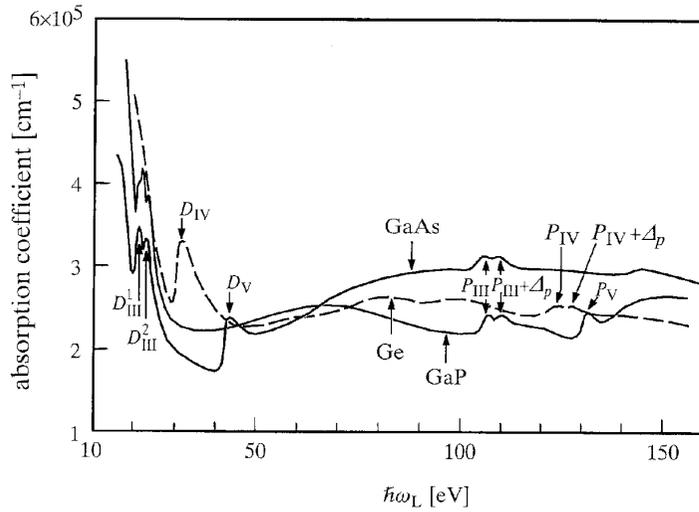
Fig. 8.2. Absorption spectra of GaP, GaAs and Ge.
