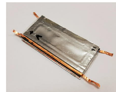
Supercapacitors with dimensions defined by the empty space inside the antenna, 3 series connected cells In one package or stacked
