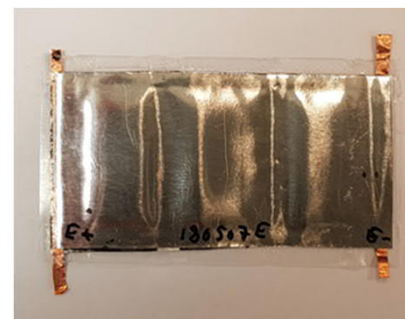
Supercapacitors with dimensions defined by the empty space inside the antenna, 3 series connected cells In one package or stacked
