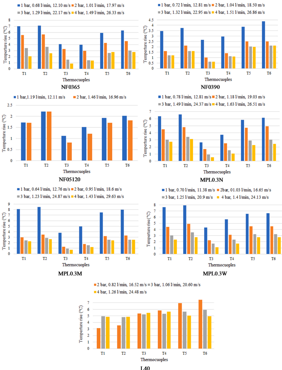
Fig. 7. Temperature rise distribution on the surface of the rectangular conductor during the operation of the nozzles under study.
