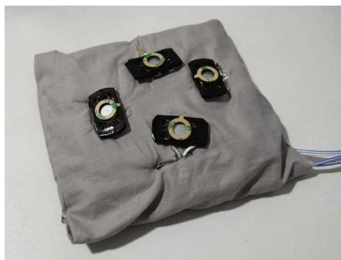
FIGURE 13. Pillow with four actuators used in the study by Köpsel et al. (2016).
